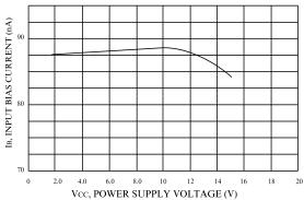
Figure 6. Input Bias Current versus Power Supply Voltage
